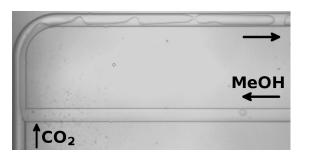
Figure 9.8: Wavy-Taylor flow regime of  $CO_2$ -MeOH mixture at P = 9.81 MPa and T = 323.6 K.
