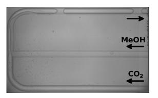
Figure 8.16: Image recorded with the CCD high-speed camera attached to the inverted microscope. Taylor flow of  $CO_2$ -MeOH, at 6.89 MPa and 305.6 K.
